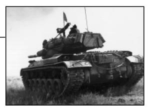
A gasoline engine limited the range of the M47, above. Most were exported. Instead, the U.S. adopted the dieselpowered M48, below.
